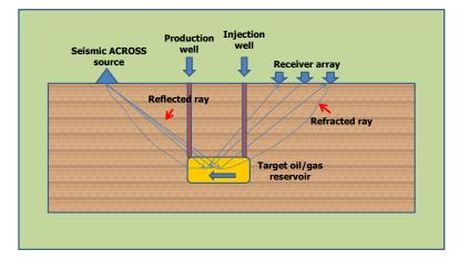
Suitable solution in a wide range of industrial and environmental applications for continuous as well as routine monitoring of CO2 injection and storage, O&G production-related changes, EOR operations, aquifer surveying, etc.
