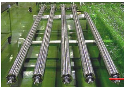
Control Rod Driving Mechanism
